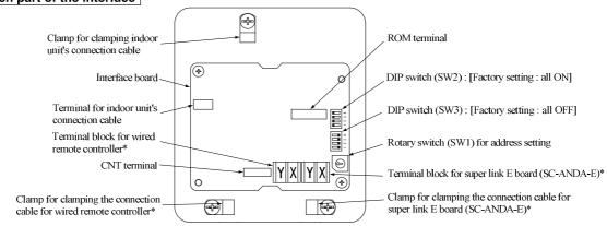
\*Either the connection cables of super link E board (SC-ANDA-E) or of wired remote controller is connectable.
